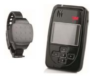
The TPTU works by attaching a Transmitter to the subject, and the Tracker is the hand held devise that receives signals from the Transmitter, thus monitoring the presence of the 'tag'.
